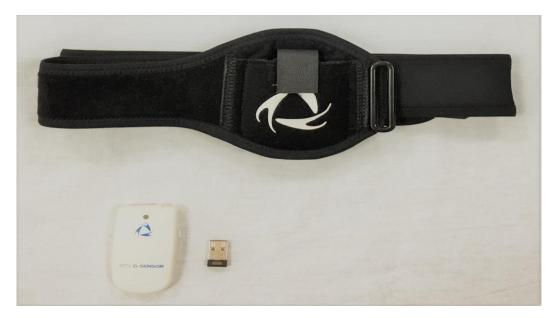
Figure 1: BTS G-WALK Tempora-Spatial wireless digital gait analysis system
