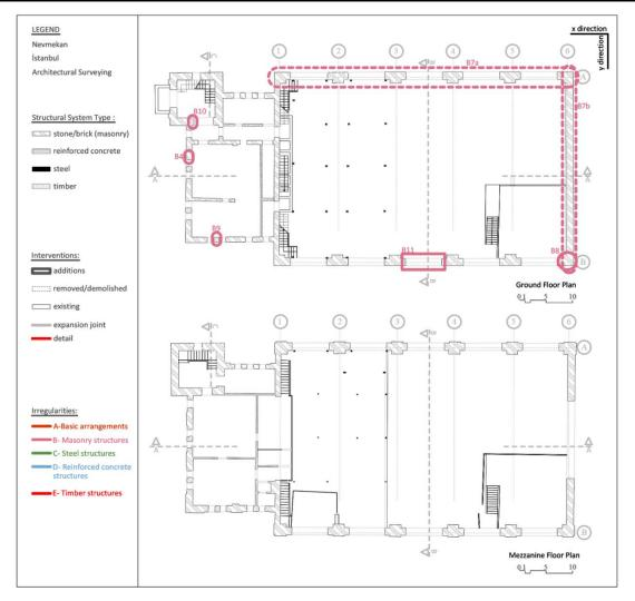
Figure 3. Üsküdar Electricity Factory architectural surveying floor plans (Adapted from Köroğlu, 2019)
