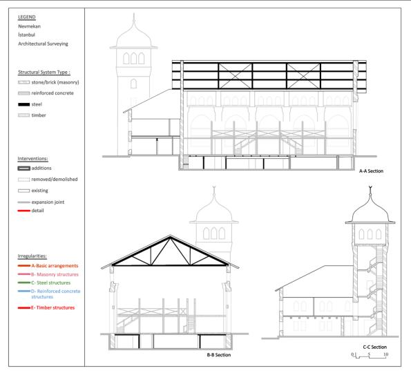
Figure 11. Nevmekan restoration project sections (Adapted from Köroğlu, 2019)
